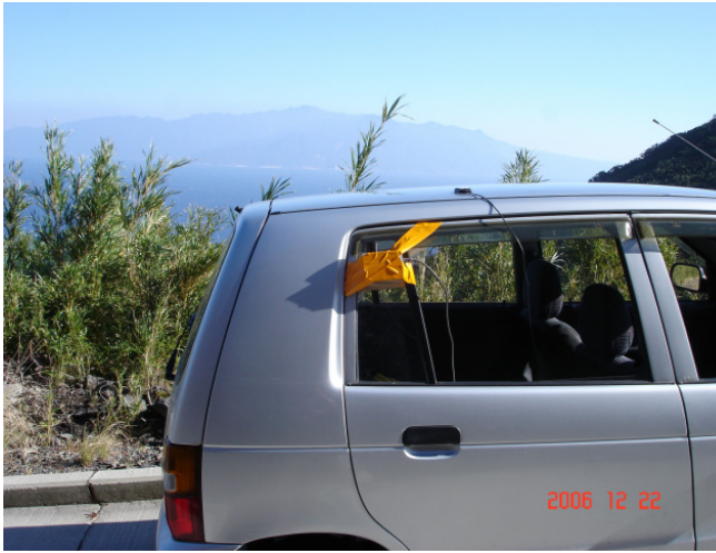
Picture 2. Snapshot of car traverse measurement at Kuchinoerabu. The GPS antenna is placed on the roof and USB2000 is attached to the door. Both data is recorded on the same PC.
