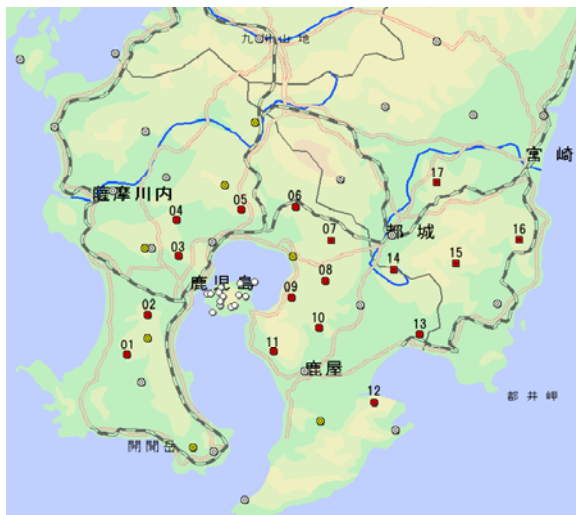
Fig. 6 Location of temporary seismic stations. Red circles and squares indicate 2Hz and 1Hz seismometers installed temporarily, respectively. Yellow and white circles around Aira caldera indicate permanent stations operated by SVRC and Hi-net stations of National Research Institute for Earth Science and Disaster Prevention, respectively.
