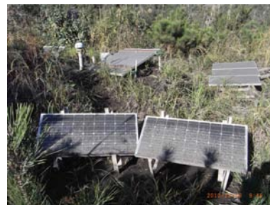
Photo 2 Solar cells employed at Gongen station. Front two panels are coated and others are not-coated. Ash fall deposit on coated panels is thinner than that on others.
